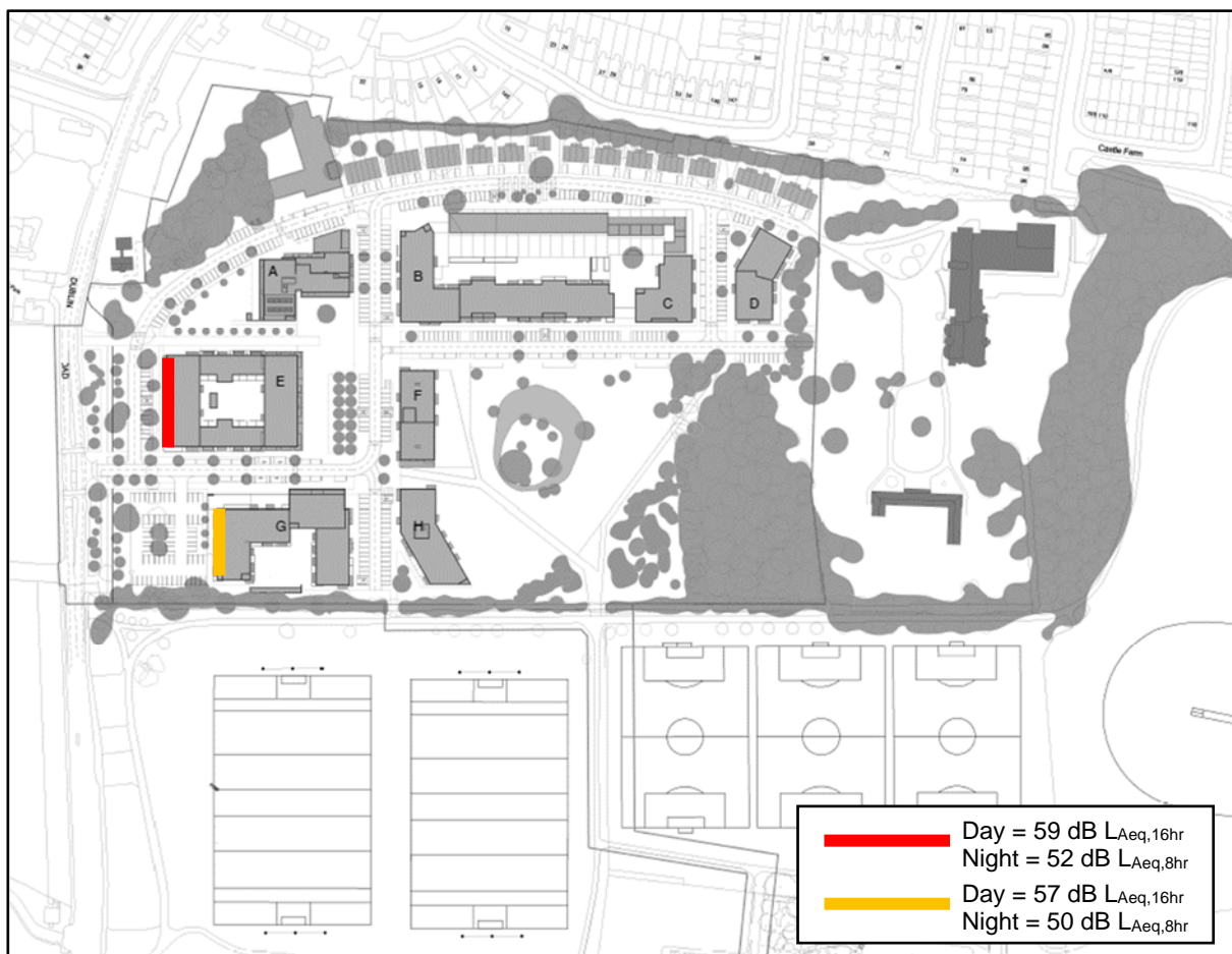
Figure 11.7 - Locations Requiring Acoustic Façade Specification
